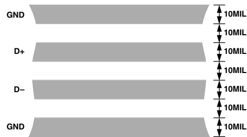
Figure 13. Arrangement of Signal Tracks
