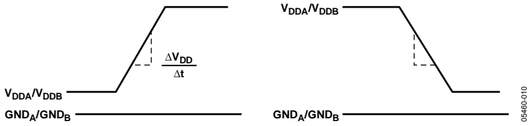
Figure 13. Transient Immunity Waveforms—Output Supplies
