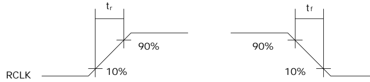
Fig. 4 Signal Rise and Fall Characteristics
