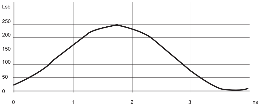
Figure 12. Reconstructed Signal for F_S = 500 Mps, F_{IN} = 250 MHz (Full Scale Input)
