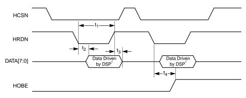
Note: <sup>\*</sup>Data is driven by the LSI403LP Digital Signal Processor (DSP).
