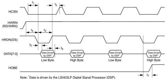
Figure 13 HPI Host Read, Motorola Mode, two 16-bit reads, 2 items in FIFO (lof=1)
