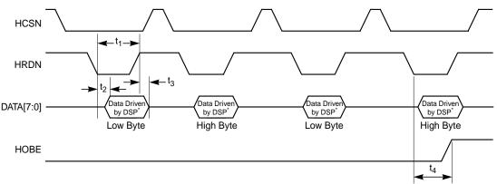
Note: <sup>\*</sup>Data is driven by the LSI403LP Digital Signal Processor (DSP).
