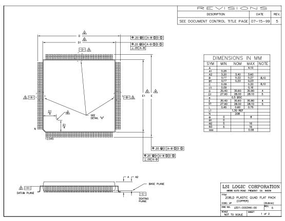
Important: This drawing may not be the latest version. For board layout and manufacturing, obtain the most recent engineering drawings from your LSI Logic representative by requesting the outline drawing for package code UP.
