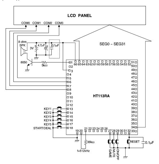
Note: The capacitor in the dotted block is recommended.
