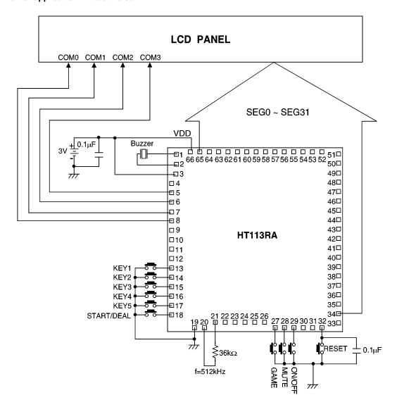
Note: The IC substrate should be connected to VSS in the PCB layout artwork.
